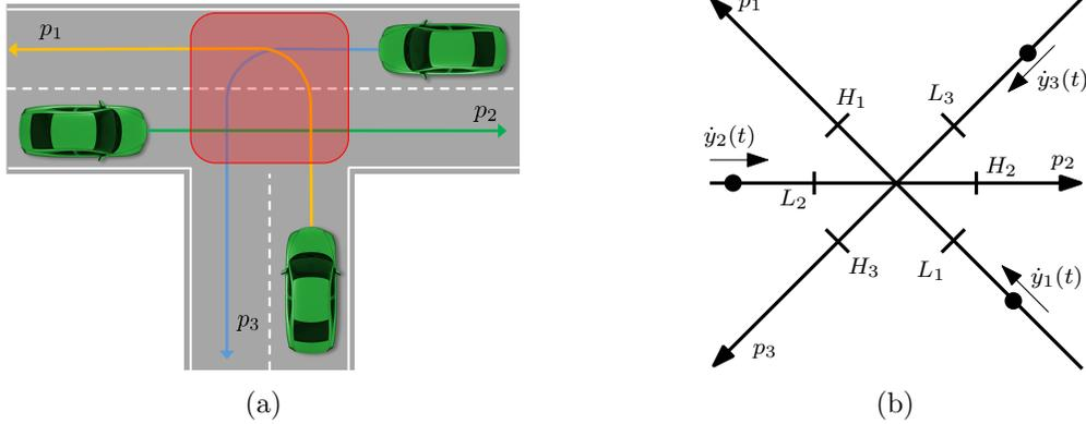
Figure 2.1: Illustration of the considered scenario: (a) A road intersection scenario with predefined paths  $p_1, p_2, p_3$ . The region where collisions can occur is marked in red, (b) The abstraction of the intersection used in modelling.
