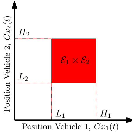
Figure 2.2: Schematic illustration of a 2D cut of the state-space in (2.6). The red area contains the infeasible state space combinations according to (2.6c) and corresponds to collisions between vehicles 1 and 2.
