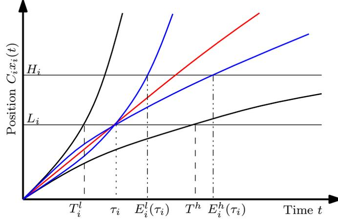
Figure 3.1: Schematic visualization of the defining elements of  $\mathcal{S}_i(x_{0,i})$ . The curved black lines represent the trajectories resulting from maximum and minimum control signal respectively. The curved blue lines show the same *given* that the entrance time  $\tau_i$  is enforced. The red line is the optimal trajectory when  $\tau_i$  is enforced.
